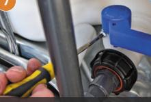
Unlock the valve lever by loosening the screw below the blue lever arm.
