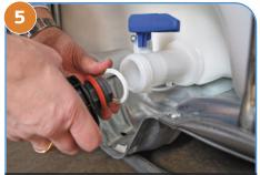
Attach the long outlet pipe to the outlet of the unit by screwing the black ring onto the thread. Ensure that the pipe is fitted with a white sealing ring.
