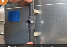
Click the top of the outlet pipe into the two holders to secure the pipe in the upright position on the front panel.
