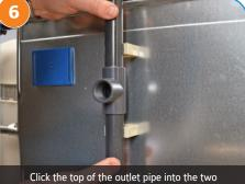
holders to secure the pipe in the upright position on the front panel.
