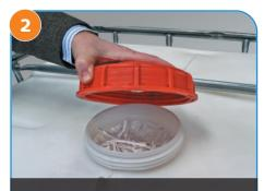
Remove red cap from the top of the unit. (Retain this cap for use during collection)
