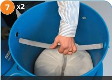
Install the securing spring clips at 90 degrees directly in contact with the filter bags to prevent floatation
