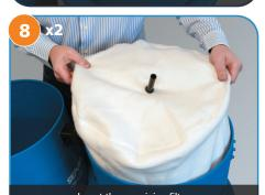
Insert the remaining filter (the one in the needle-felt bag) with the connecting tube uppermost.
