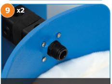
Screw the inlet connector (Reducing Bush) into place tightly.
