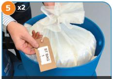
Lower the filter bag 1 into the separator body, settling it down gently, and ensuring it is in contact with the side wall.
