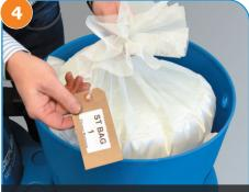
Lower the filter bag 1 into the separator body, settling it down gently, and ensuring it is in contact with the side wall.
