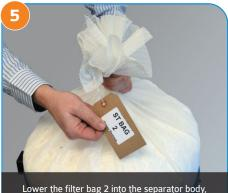
Lower the filter bag 2 into the separator body, settling it down gently on top of filter bag 1.
