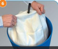
Insert the second filter bag (needle-felt bag with black inlet tube) and rest it on top of the retainers.
