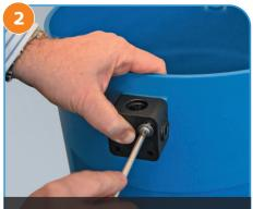
Fit the inlet block to your chosen side using the screws provided. (Extra blocks can be purchased if required.)
