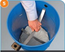
Insert the metal retainer(s) with bent ends facing upwards. Slide down until it touches the top of the filter bag. DO NOT compress the filter bag.
