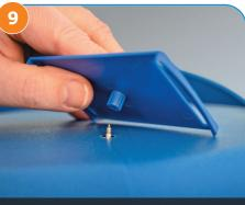
Assemble and attach the service life indicator to the lid of the unit using the pre-drilled hole. See overleaf for more detail.
