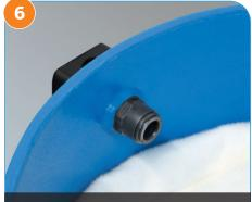
Screw the inlet connector (Reducing Bush) into place tightly.
