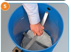
Insert the metal retainer(s) with bent ends facing upwards. Slide down until it touches the top of the filter bag. DO NOT compress the filter bag.
