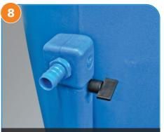
Attach the twist off Grab Tap to the test point. Attach your outlet hose to the nipple above. Fill unit with water and check for leaks.
