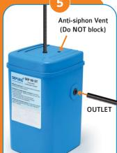
Connect tube into outlet fitting and feed to drain (side). Ensure a steady fall from outlet point to drain with no kinks or tight bends.
