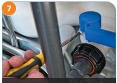
Unlock the valve lever by loosening the screw below the blue lever arm.
