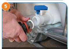
Attach the long outlet pipe to the outlet of the unit by screwing the black ring onto the thread.
