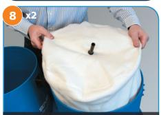
Insert the remaining filter (the one in the needle-felt bag) with the connecting tube uppermost.
