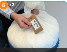
Lower the filter bag 2 into the separator body, settling it down gently on top of filter bag 1.
