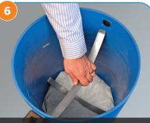
Install the securing spring clips at 90 degrees directly in contact with the filter bags to prevent floatation.
