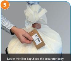
settling it down gently on top of filter bag 1.
